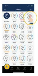
1. From the Lights page, do an extended press and hold on a light's icon to open the Light Dimming settings page.
